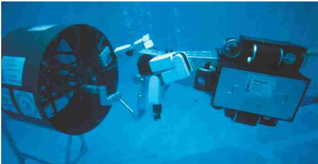
Figure 5 – RANGER NBV-I in Testing with Dexterous and Grapple Arms
