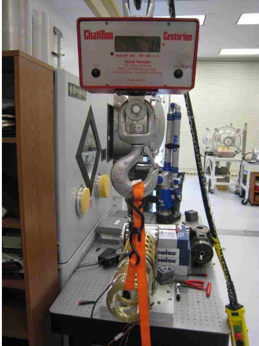
Figure 26 – Crane Scale Test Setup for Current/Torque Test
