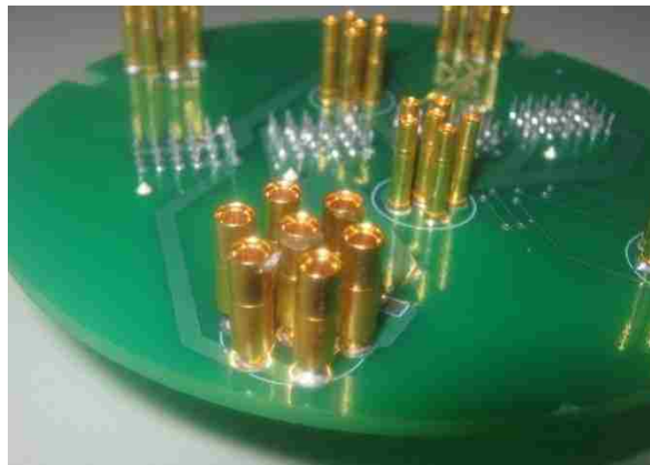
Figure 18 - SAMURAI Penetrator Board with Hypertronics Penetrator Pins
