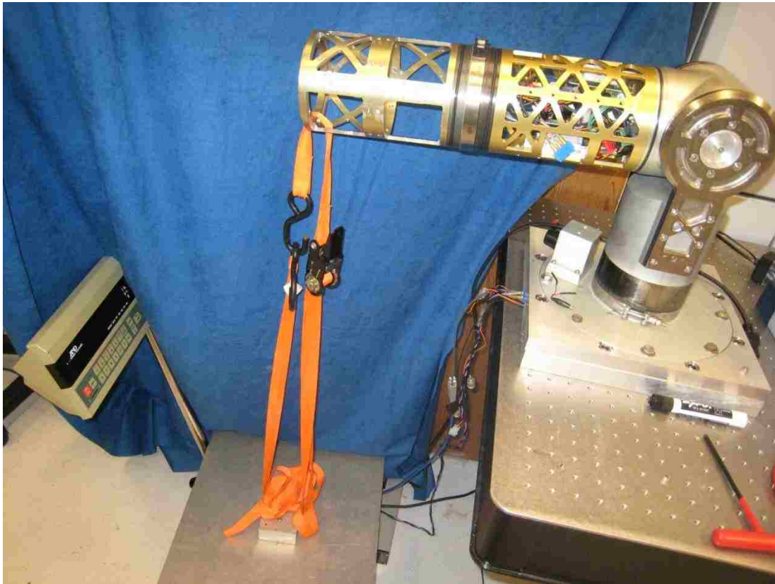
Figure 25 - Electronic Balance Test Setup for Current/Torque Tests
