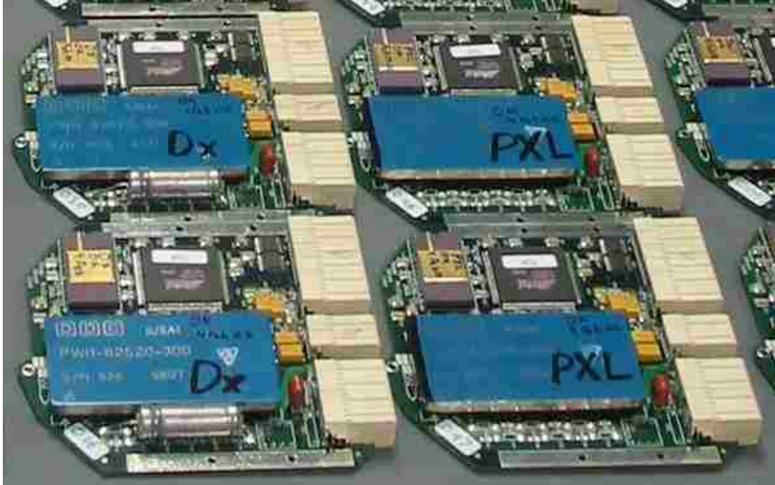
Figure 8 - RTSX/NBV-II Motor Driver Boards
